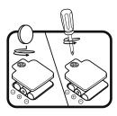
4. Replace the battery cover and tighten the screw to secure.
